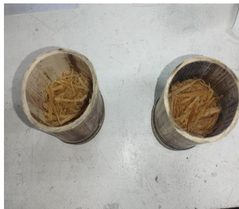
Figure 13. Layering the Bamboo in the Mold
